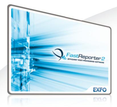
Consolidated data management and post-processing tool designed to increase the reporting productivity for connector endface inspection and all types of optical-layer testing: optical link mapper (iOLM), OTDR, ORL, loss, PMD and chromatic dispersion (CD)
